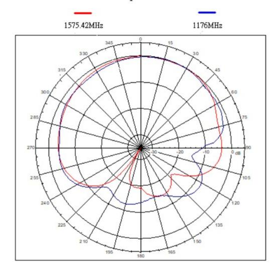
PS: Total Gain = Passive Pattern Gain + LNA Gain - cable loss (1.1dB/m)
