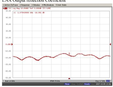
The S-parameters of LNA in the condition of -40 dBm input power.
